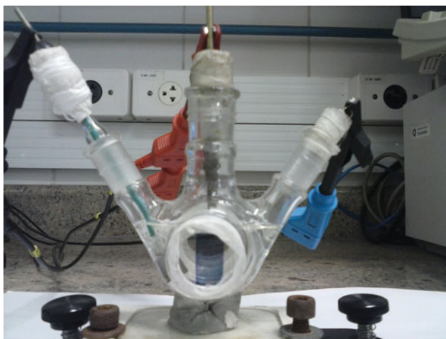
Figure 1. Three-electrode electrochemical cell with two quartz windows and WO 3 blue colored thin film inside the cell.
